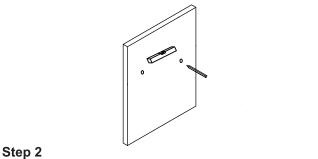
Mark the holes position with pencil, make sure the holes are level.
