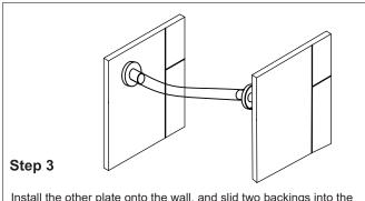
Install the other plate onto the wall, and slid two backings into the plate, make sure the 2 holes on the top.
