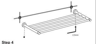
Slide the accessory onto the backing plates and tighten the set screws using Allen key provided.
