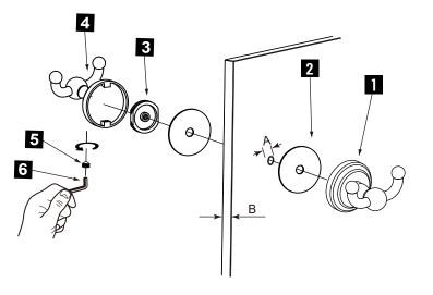
2.Clear Gasket x 2 3.Fixing Bracket x 1 4.End Cap x 1 5.Set Screw M5 x 1 6.Allen Key 2.5mm x 1
