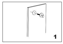
Install the hook (bolt) throught the glass hole, make sure the rubber gaskets are between knob&glass.
