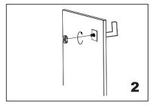
Screw in the fixing bracket into the knob bolt.
