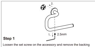
plate. Position the accessory against the wall and mark outline with pencil.
