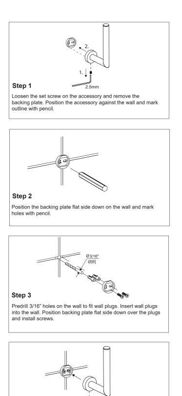
2.5mm Slide the accessory onto the backing plate and tighten the set
