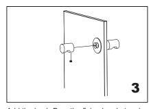
Add the knob-B on the fixing bracket,make sure the set screw hole in the bottom.
