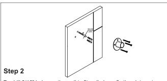
Predrill 3/16" holes on the wall to fit wall plugs, fix the plate onto the wall, make sure the post hole on the top.
