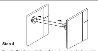
Press the 2 backings onto the plates, make sure the backing would not fall off from the plate.
