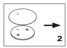
Tear off the double-sided adhensive tape on part 5 (heavy bottom).
