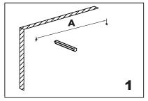
Mark (on the wall) locations of plugs through mounting plate using a pencil, refer to Fig.1
