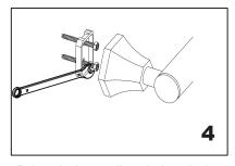
Driver bolt nut directly into holes
