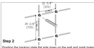
Position the backing plate flat side down on the wall and mark holes with pencil.
